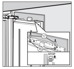
Open the door and hang the custom door with the mounting frame over the threaded bolts <sup>(6)</sup>.
